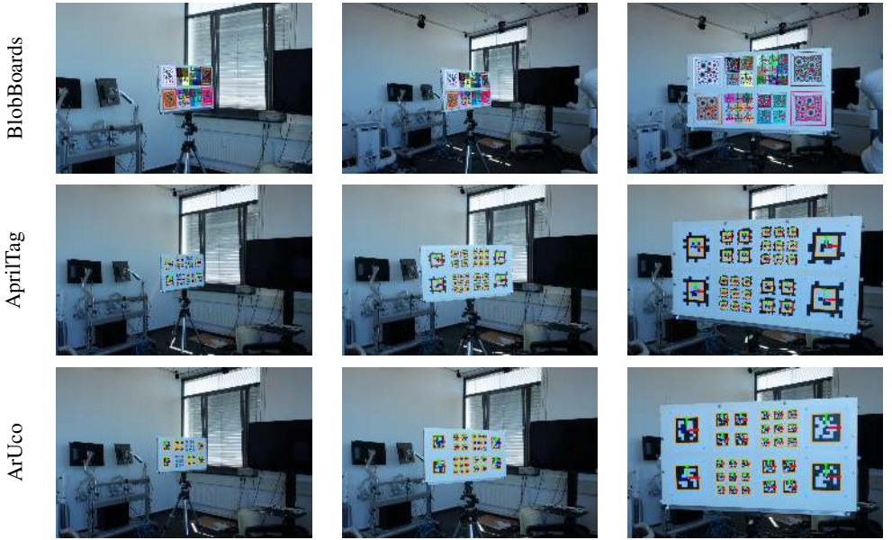
Figure S1: Experimental setup. BlobBoards, AprilTag, and ArUco are mounted on matched rigid panels containing 30 markers at three physical scales: 18 small, 8 medium, and 4 large. The panel is observed at varying distances and obliquities while its 6-DoF pose is tracked by motion capture. Estimated board coordinate frames are overlaid; for BlobBoards, the reference pattern is additionally projected under the recovered pose.
