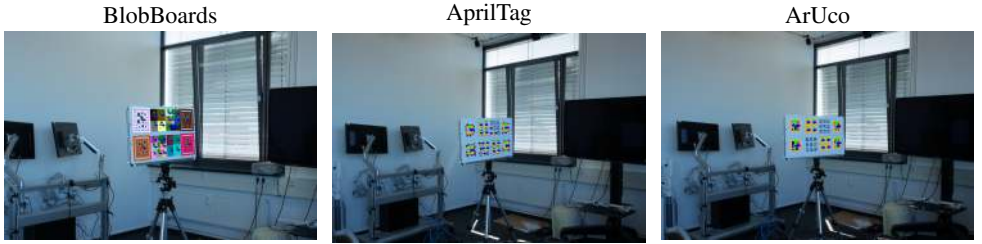
Figure 5: Experimental setup, one capture per marker type. Each type is mounted on a matched rigid panel carrying 30 markers at three physical scales (18 small, 8 medium, 4 large), observed while motion capture tracks the panel’s 6-DoF pose. Estimated board frames are overlaid; for BlobBoards the reference pattern is additionally projected under the recovered pose. Further captures are in supplementary fig. S1.
