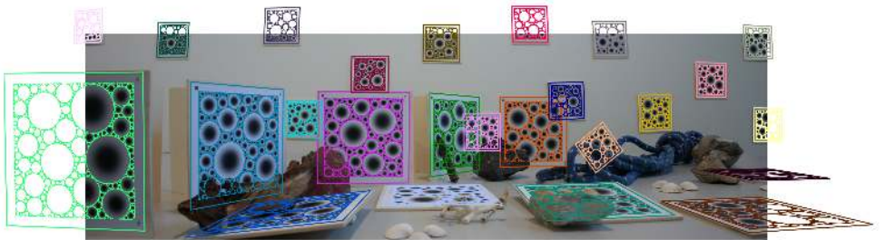
Figure 1: All 25 BlobBoards in the image are detected, identified, and registered against a 50-board gallery, so 25 of its entries are absent confusers, and identification is still perfect. Colour distinguishes detections; the overlaid pattern shows registration accuracy across large variations in scale, distance, and obliquity.
